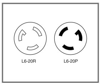
**Figure 6.** NEMA-style L6-20 plug and receptacle.
